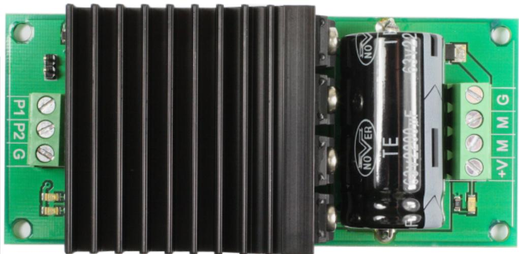
**Note - There is no fuse on the PCB. You should provide a 25/30A fuse in line with the +v battery terminal.**
